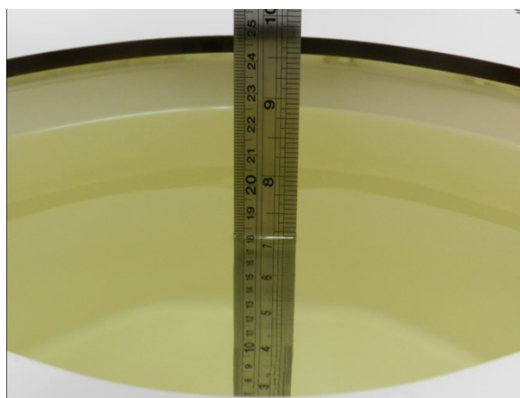
Fig 10.2 Photo of Liquid Height for Body SAR
