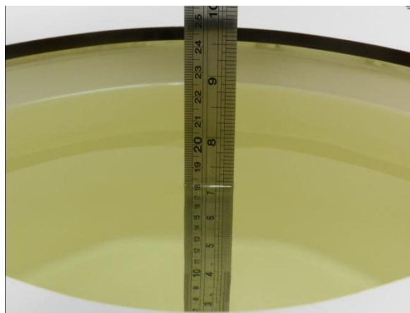
Fig 10.2 Photo of Liquid Height for Body SAR
