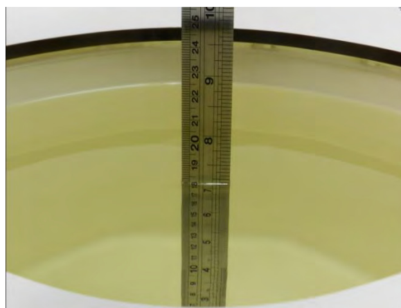
Fig 10.2 Photo of Liquid Height for Body SAR
