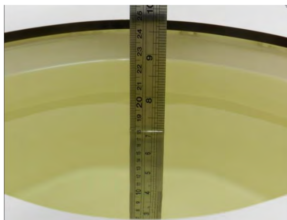
Fig 10.2 Photo of Liquid Height for Body SAR
