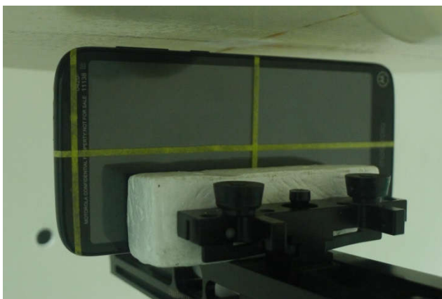
Right Side, Test Separation 5 mm
