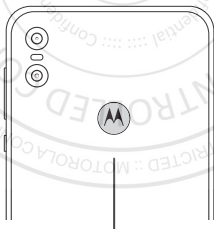
Fingerprint Sensor Press to unlock.
