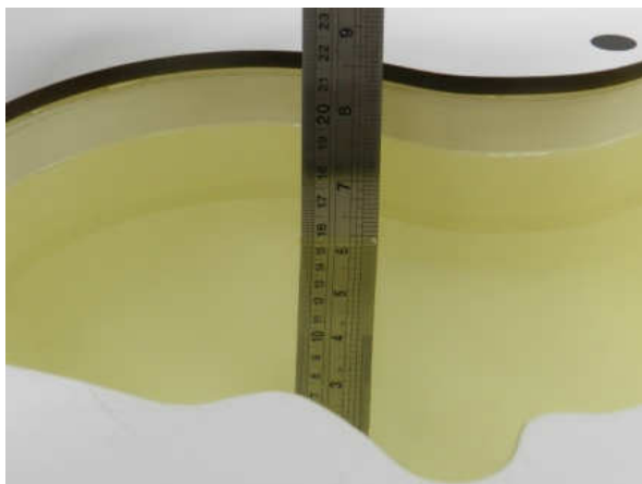
Fig 11.1 Photo of Liquid Height for Head SAR
