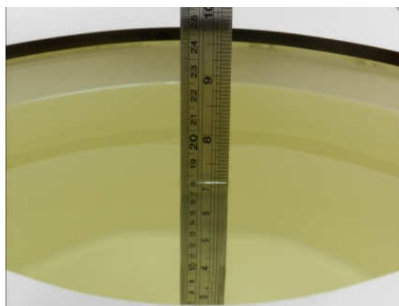
Fig 11.2 Photo of Liquid Height for Body SAR
