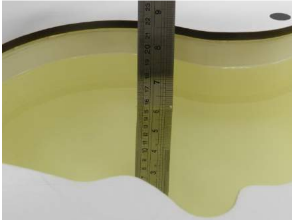
Fig 10.1 Photo of Liquid Height for Head SAR
