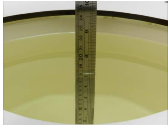
Fig 10.2 Photo of Liquid Height for Body SAR
