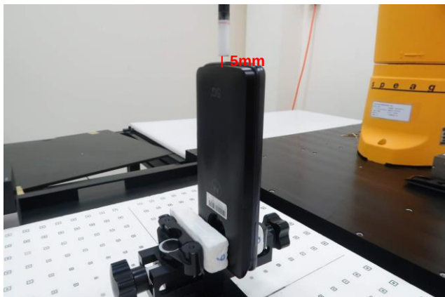
Bottom Side, Probe sensor to EUT surface distance 5mm
