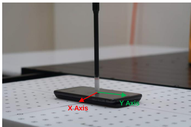
Front, Probe sensor to EUT surface distance 2mm
