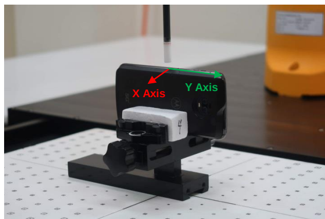
Right Side, Probe sensor to EUT surface distance 5mm
