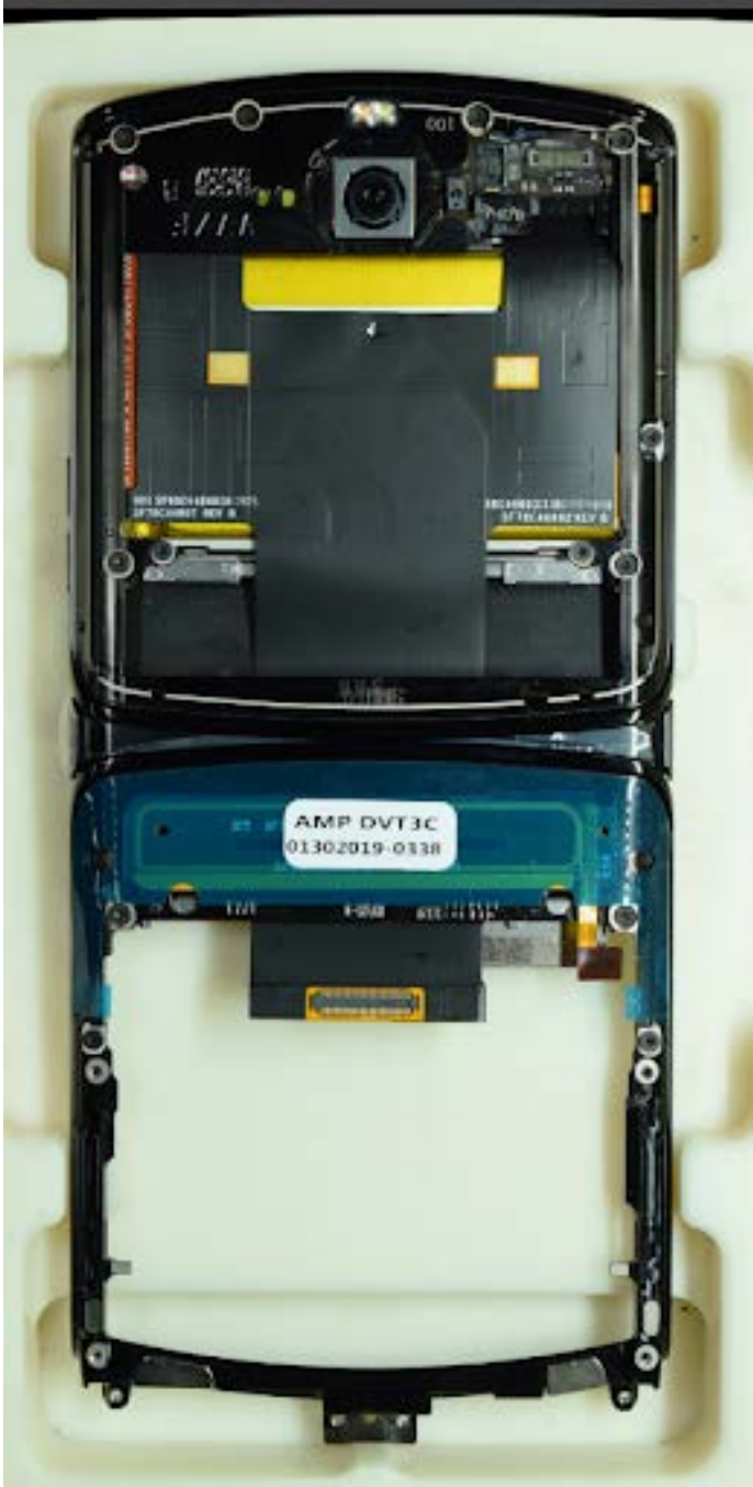
Photograph 9-7: Rear Housing with PCB / Internal Battery
