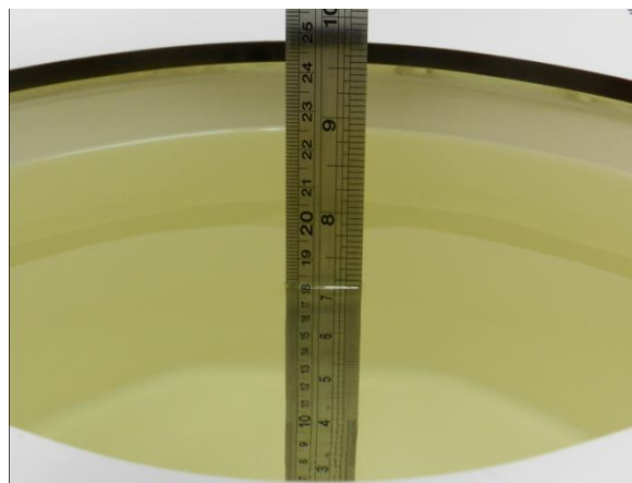
Fig 11.2 Photo of Liquid Height for Body SAR
