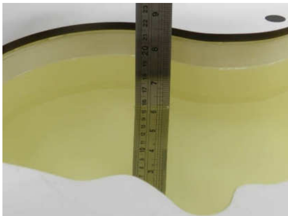
Fig 10.1 Photo of Liquid Height for Head SAR
