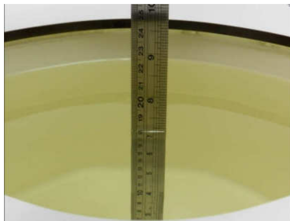
Fig 10.2 Photo of Liquid Height for Body SAR
