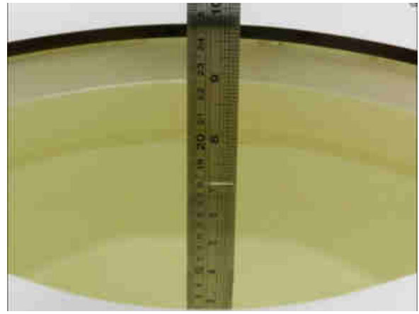
Fig 10.2 Photo of Liquid Height for Body SAR
