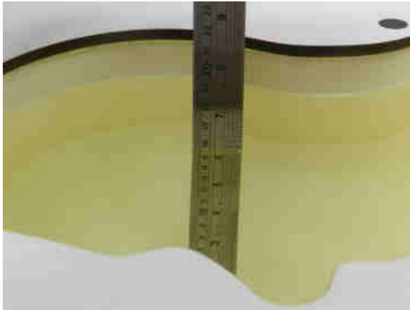
Fig 10.1 Photo of Liquid Height for Head SAR
