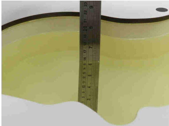
Fig 11.1 Photo of Liquid Height for Head SAR
