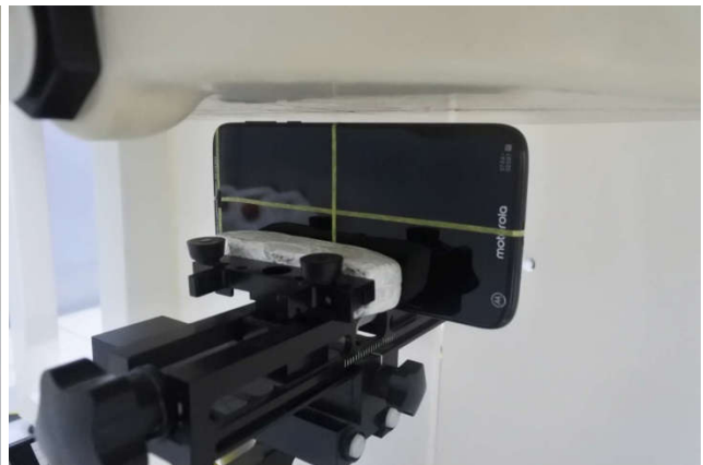
Right Side, Test Separation 5 mm
