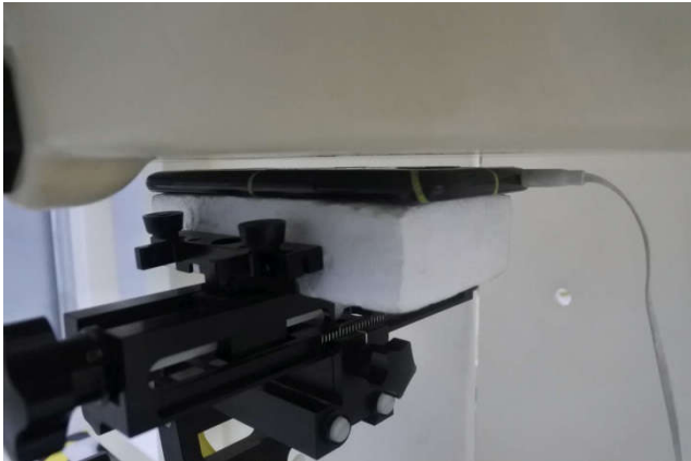
Back with handset, Test Separation 5 mm
