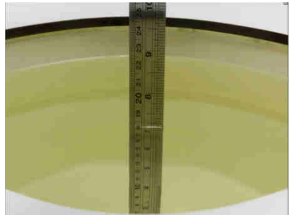
Fig 10.2 Photo of Liquid Height for Body SAR
