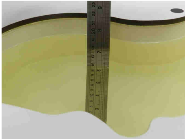
Fig 10.1 Photo of Liquid Height for Head SAR
