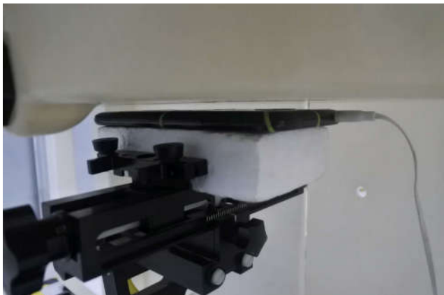
Back with handset, Test Separation 5 mm
