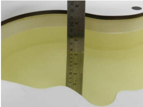
Fig 10.1 Photo of Liquid Height for Head SAR
