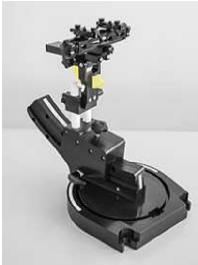
Mounting Device for Hand-Held Transmitters
