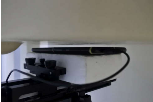
Front with handset, Test Separation 5 mm
