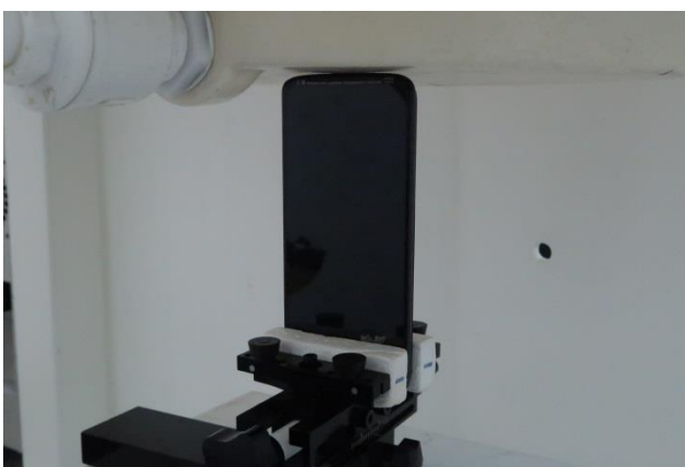
Bottom Side, Test Separation 0 mm
