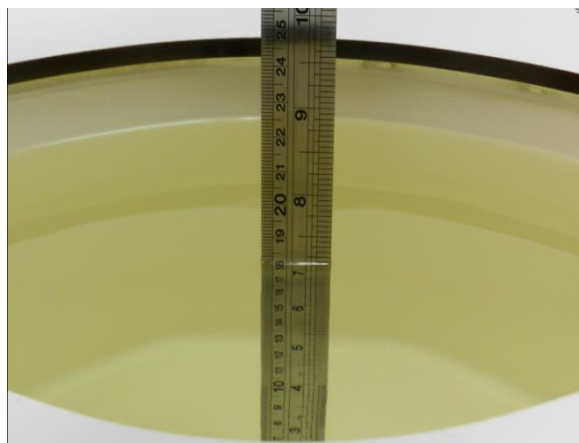
Fig 11.2 Photo of Liquid Height for Body SAR
