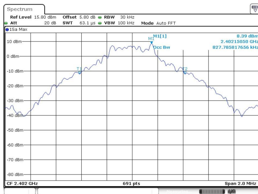
99% Occupied Bandwidth Plot on Channel 00
