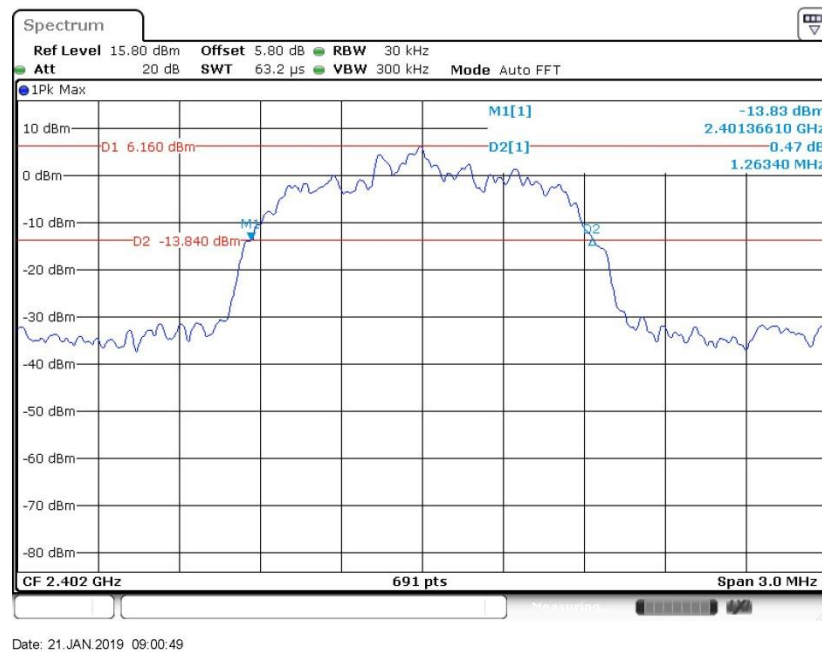
20 dB Bandwidth Plot on Channel 00
