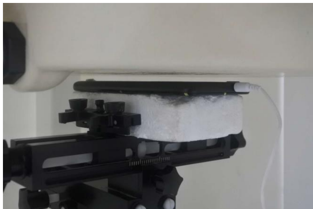
Back with handset, Test Separation 5 mm
