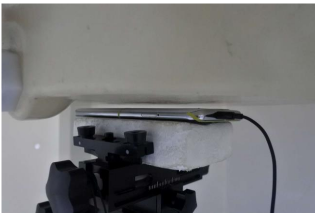
Back with handset, Test Separation 5 mm
