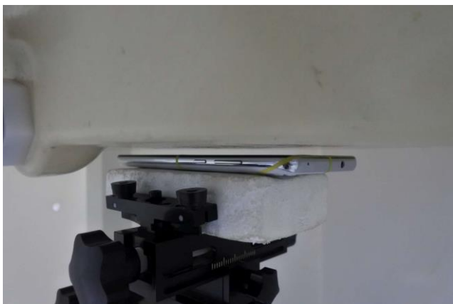
Front, Test Separation 5 mm
