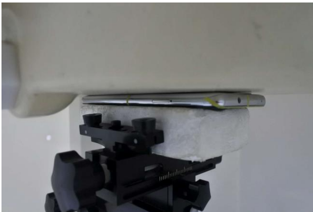
Back, Test Separation 0 mm
