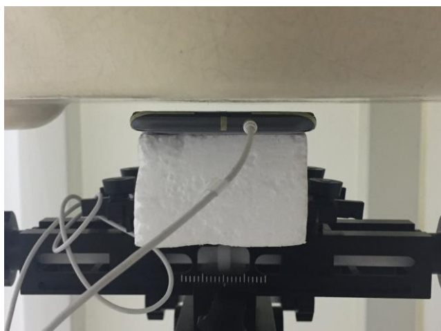
Front with headset, Test Separation 5mm
