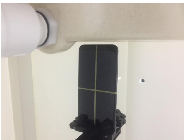
Bottom Side, Test Separation 5 mm
