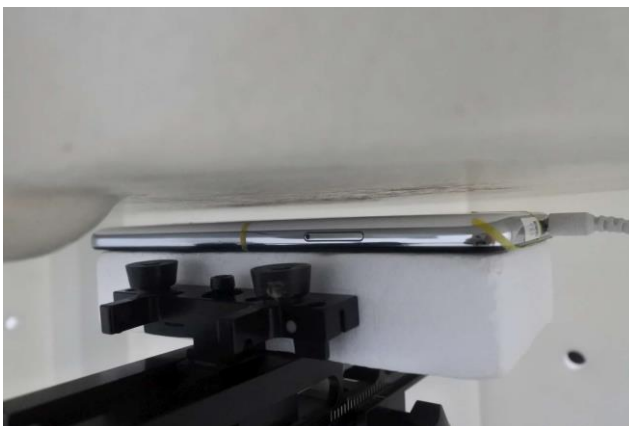
Back with handset, Test Separation 5 mm
