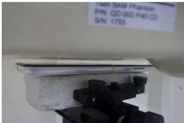
Front, Test Separation 5 mm
