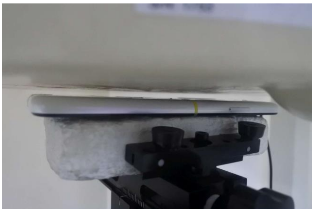
Back with handset, Test Separation 5 mm
