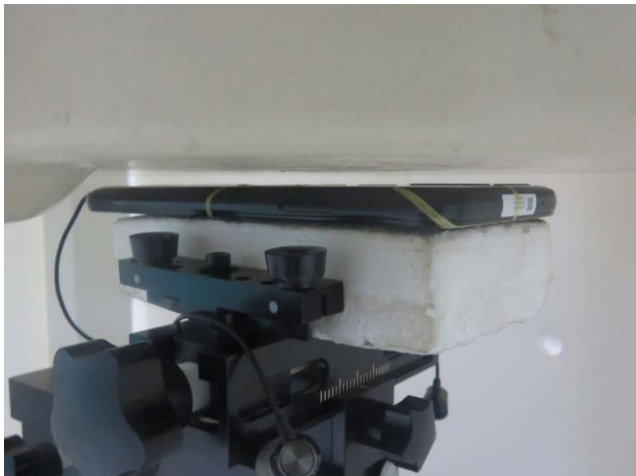
Back with handset, Test Separation 5 mm
