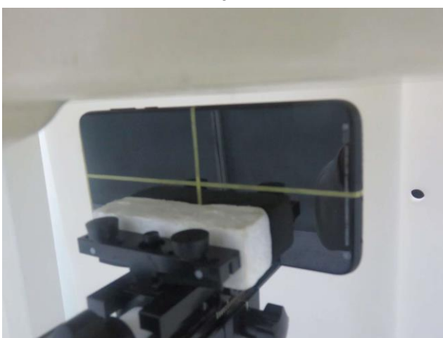
Right Side, Test Separation 5 mm
