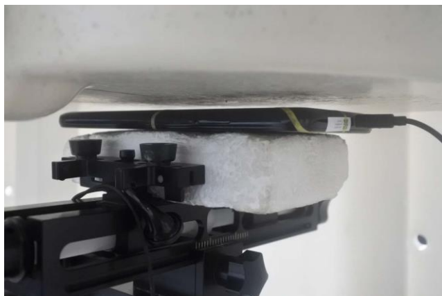
Back with handset, Test Separation 5 mm
