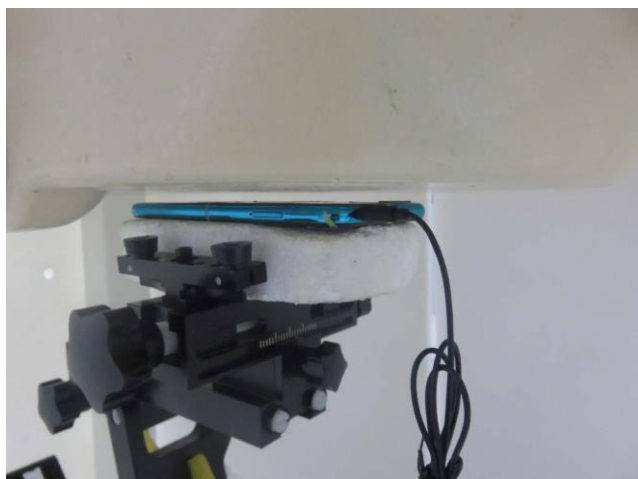
Back with headset, Test Separation 5mm
