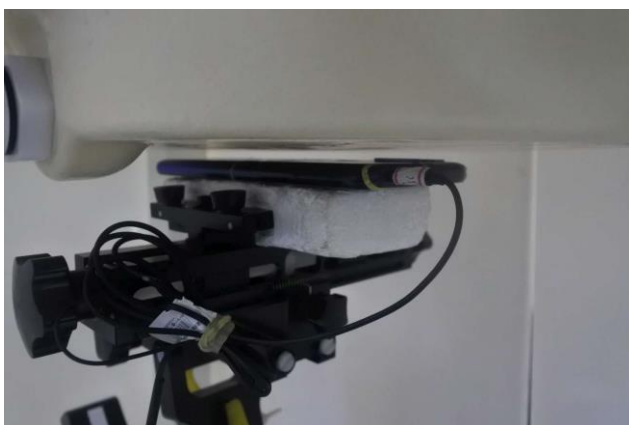
Back with handset, Test Separation : 5 mm
