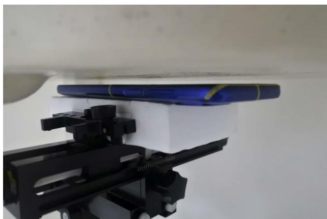
Front, Test Separation 5 mm
