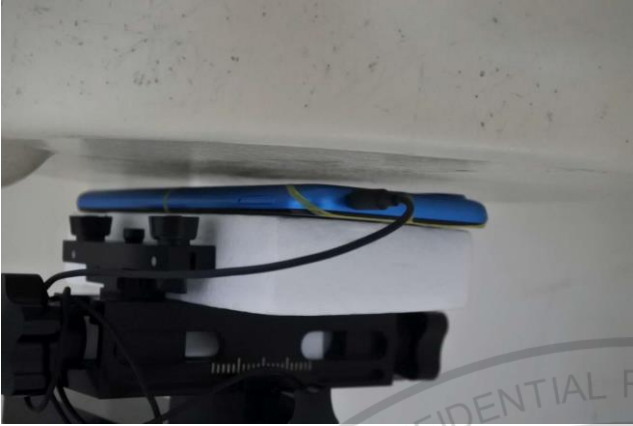
Back with Headset, Test Separation 5 mm
