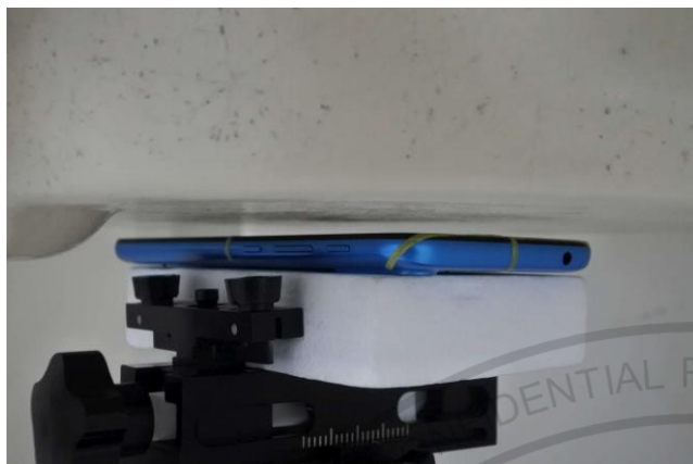
Front, Test Separation 5 mm
