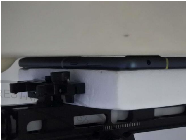
Back, Test Separation 0 mm
