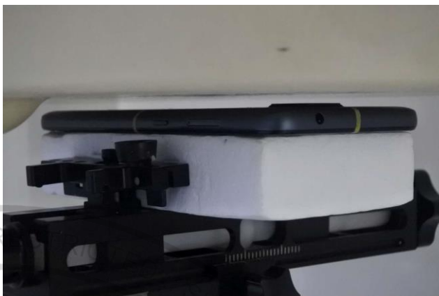
Back, Test Separation 5 mm
