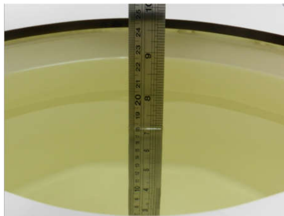
Fig 10.2 Photo of Liquid Height for Body SAR
