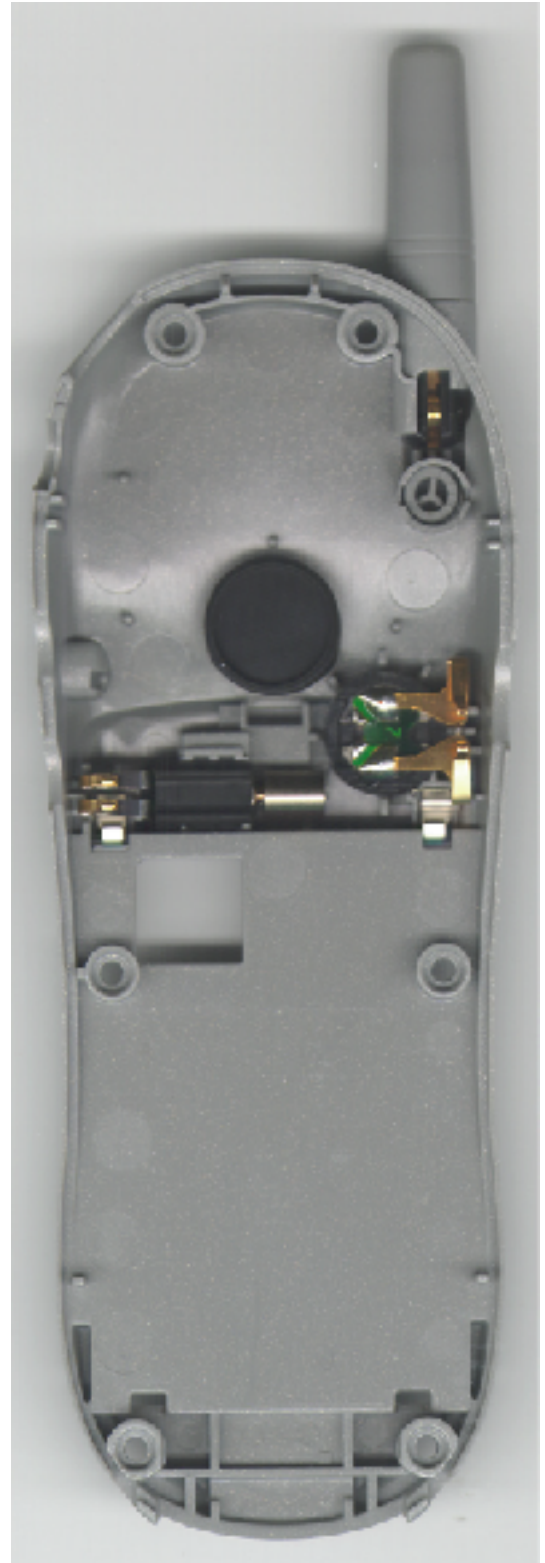
Rear Housing Internal View
