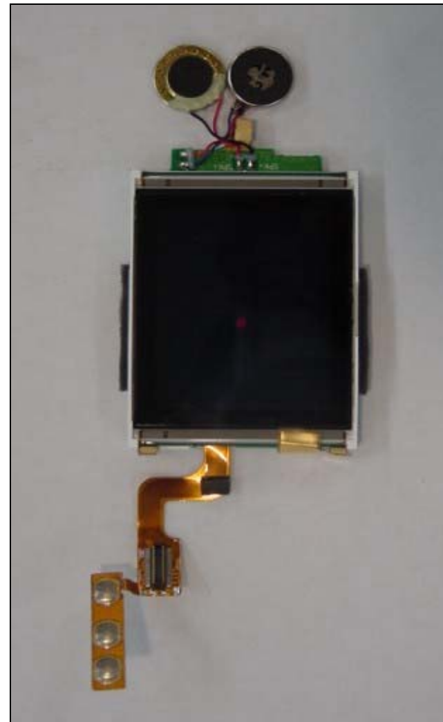
Display Board Front View
