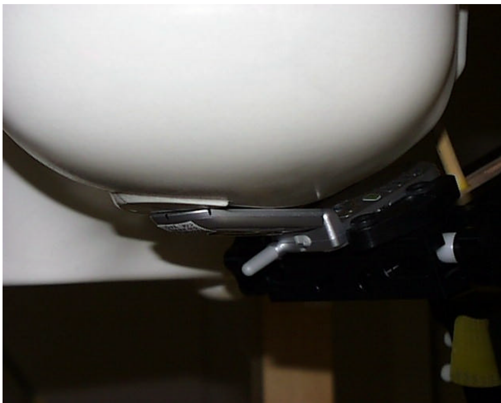
Figure 19. Phone Against head phantom (15°Tilt) with Antenna Retracted (Back View)
