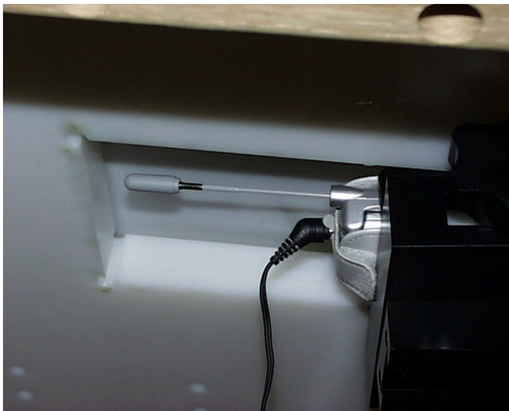
Figure 10. Phone under a flat phantom with head set attached (Antenna Extended)
