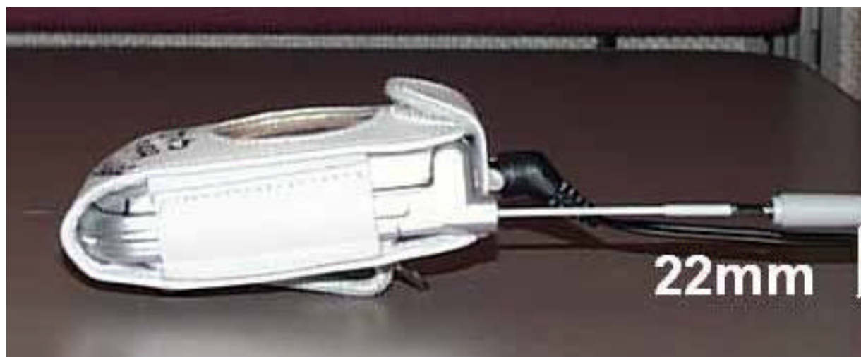
Figure 12. Distance from the base of the antenna to the flat base
