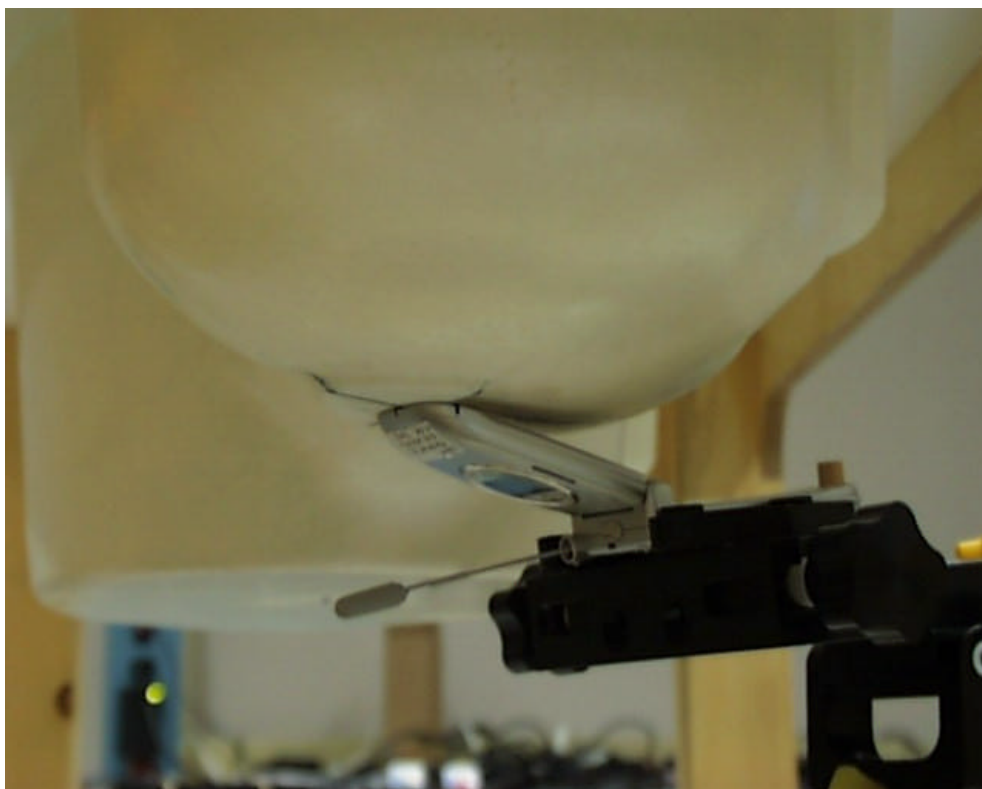
Figure 18. Phone Against head phantom (15°Tilt) with Antenna Extended (Back View)
