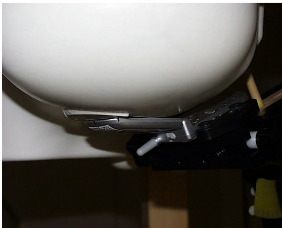
Figure 15. Phone Adjacent to head phantom with Antenna Extended (Back View)
