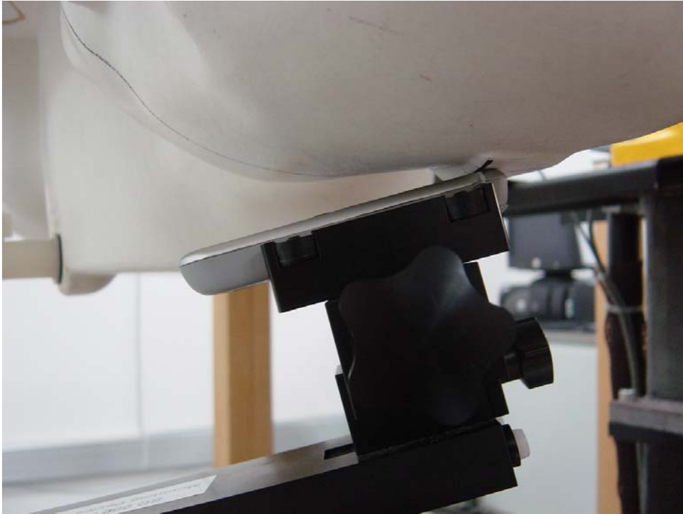
Figure 5. Phone Against the Head Phantom (15°Tilt)
