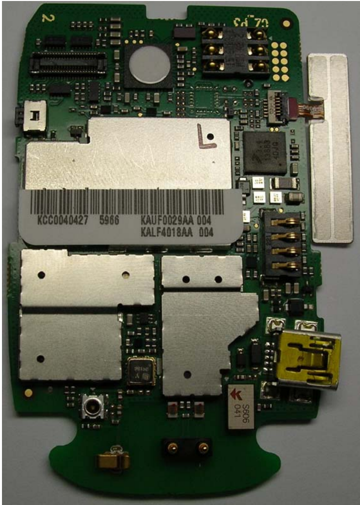
Main Board(shield on)
