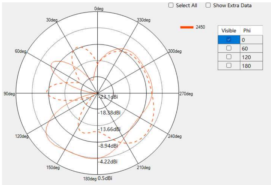
Phi=0° , Left Ear 2D Antenna Pattern, unit: dBi
