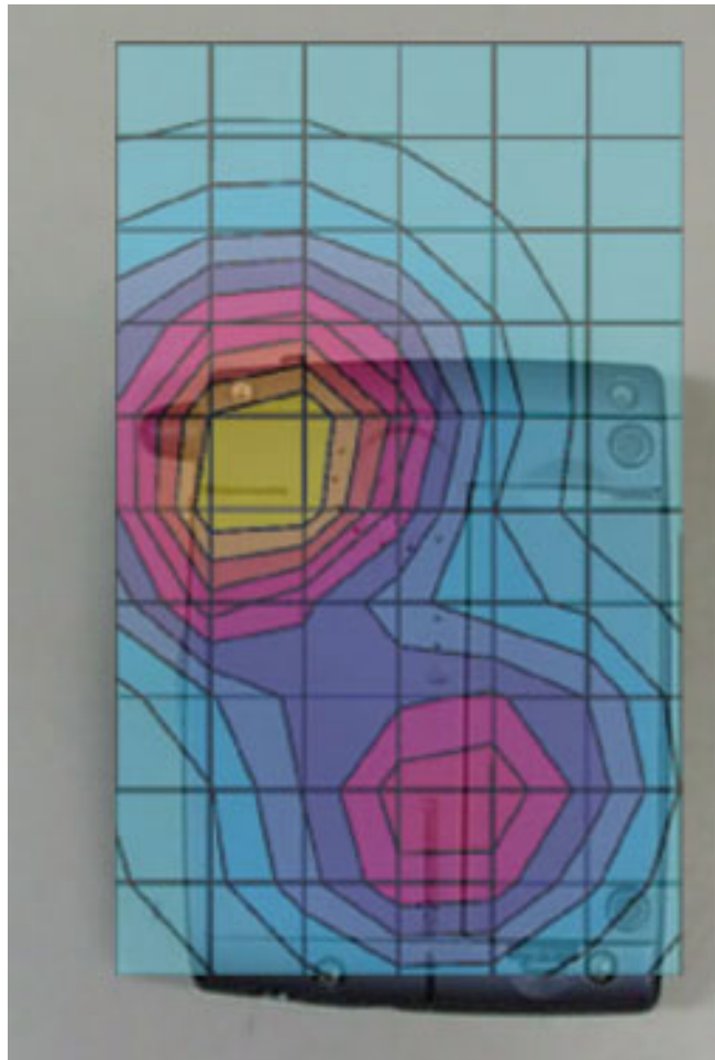
Figure 2. Typical Body Worn Contour Plot Overlaid on Bottom of Phone.
