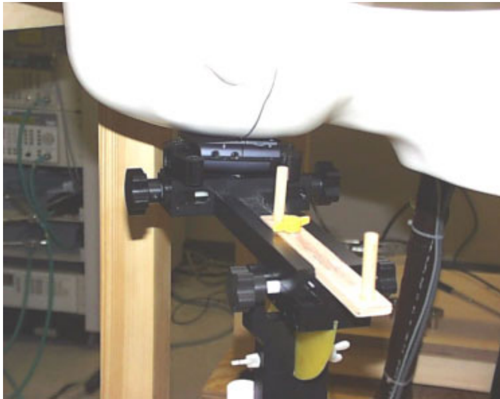
Figure 8. Phone in Cheek Touch Position with Speaker and Microphone Placed Against Phantom Head.
