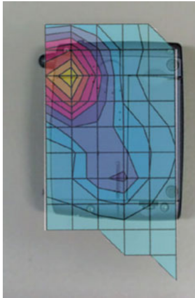
Figure 1. Typical Head Adjacent Contour Plot Overlaid on Bottom of Phone
