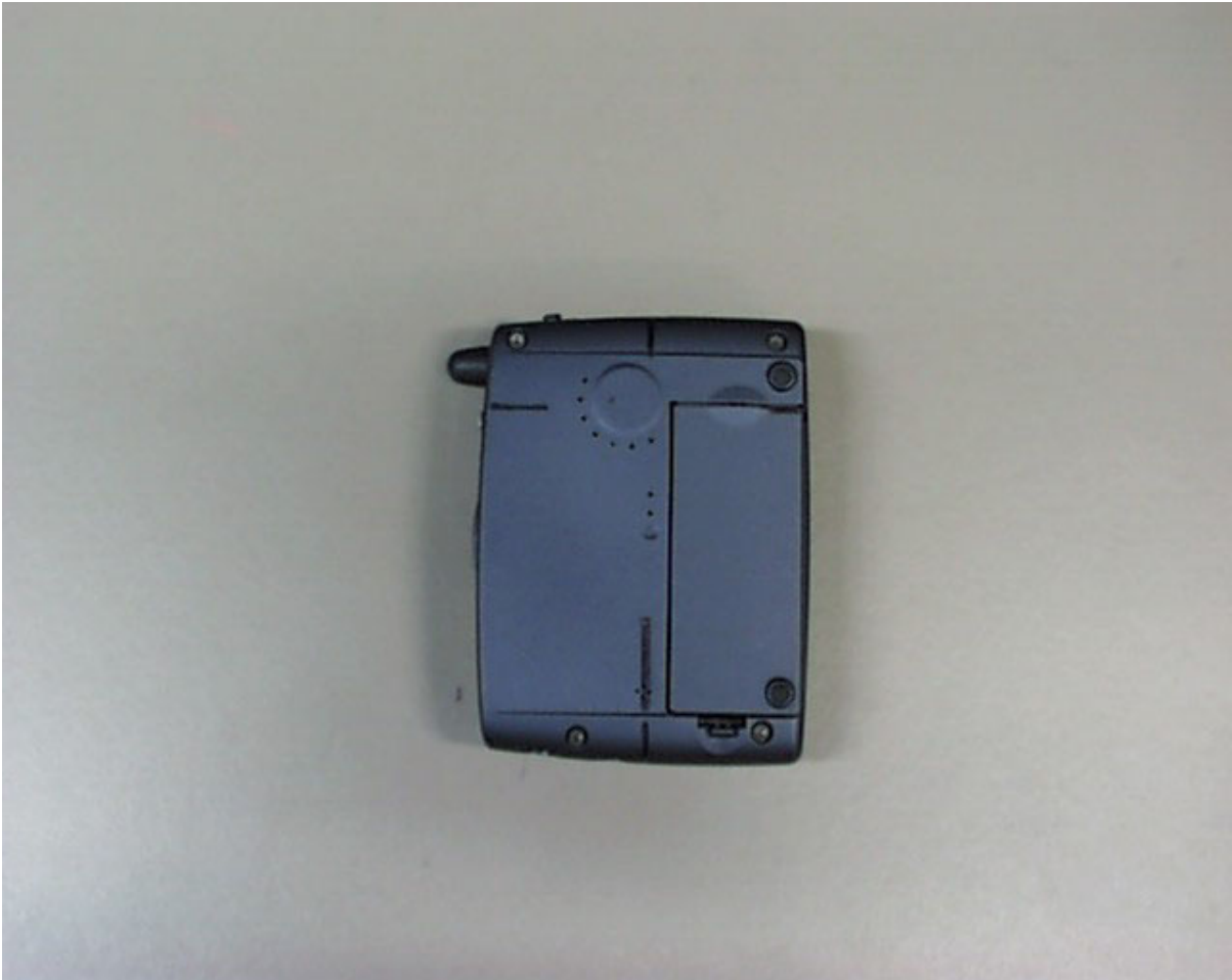
Figure 3. Bottom of Phone showing Speaker and Microphone
