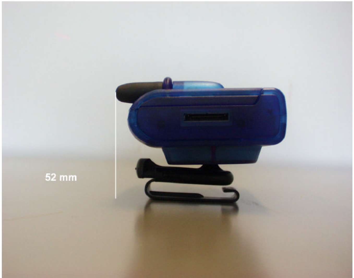
Figure 6. Distance of the Antenna from the Flat Phantom
