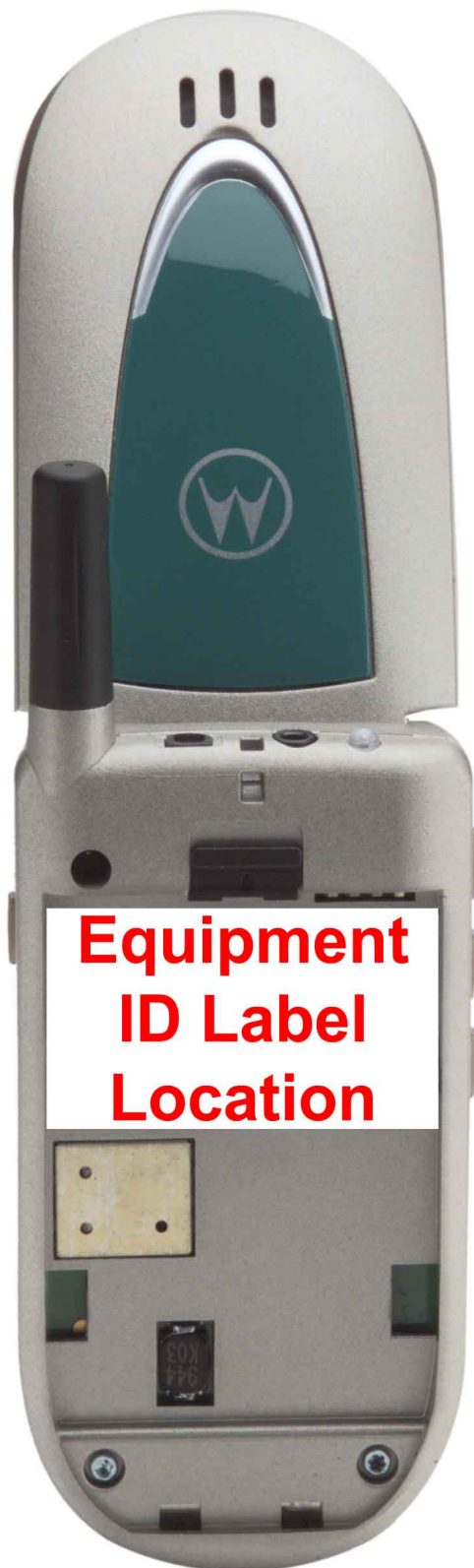
Rear View, with Battery Removed to Show Equipment ID Label
