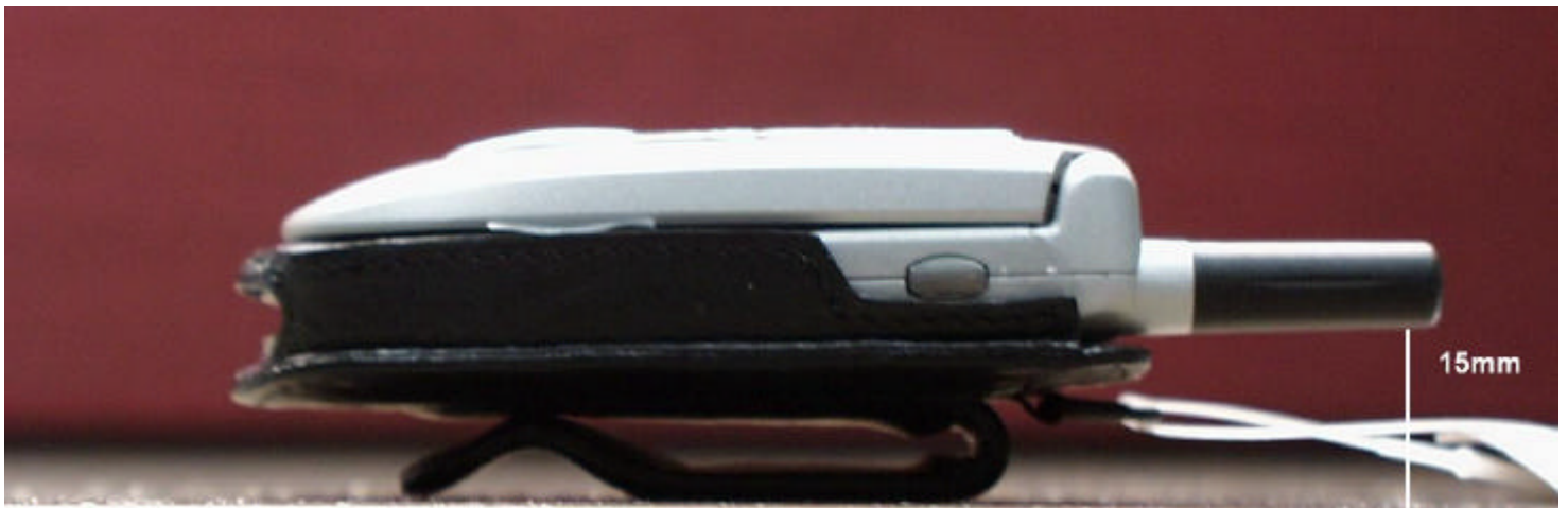
Figure 6. Distance Provided by Body-worn Accessories
