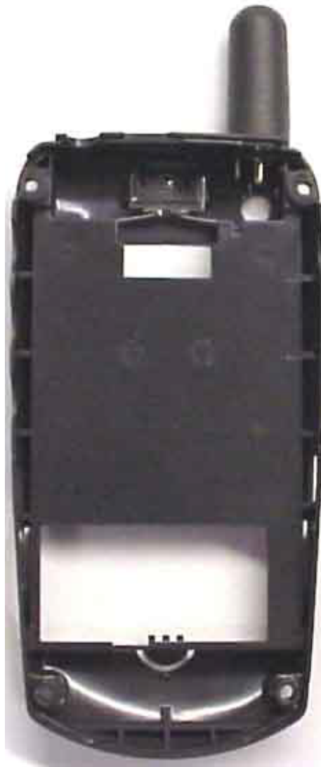
Rear Housing Internal View
